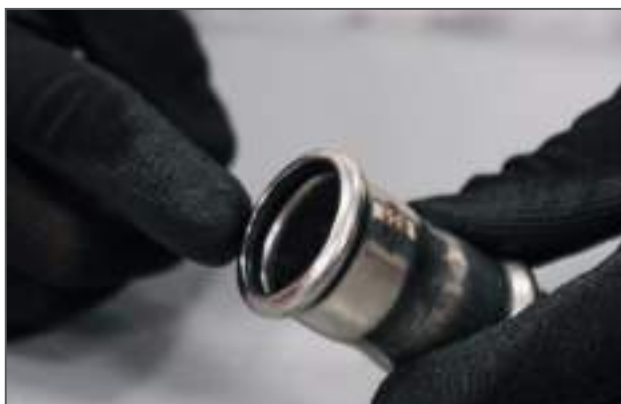
Controllo O-ring / Checking the sealing ring
